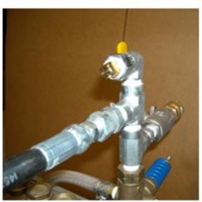
3/8" x 1" Threaded Pipe And Cap, Or Beveled Plug Note Swivel Fitting Has An Insert So Plug/Pipe Needs Bevel
